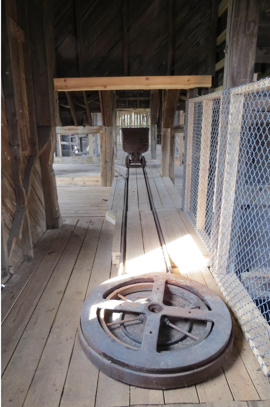
Right of Way mine – No. 2 shaft – Part of turntable mechanism used to turn ore cars before being dumped if dump door is facing wrong direction. (Track to ore bin is left of ore car) Allan Stacey©
