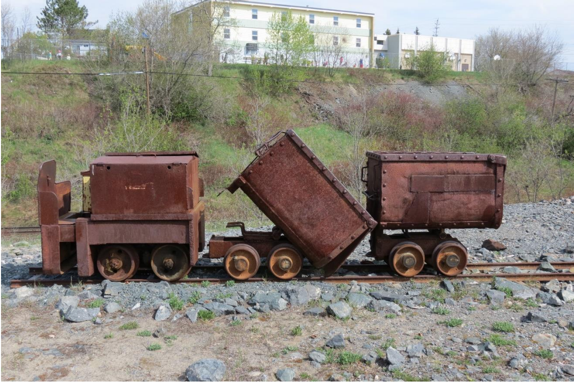
Right of Way mine – Battery trammer & two ore cars, one in dumping position. Allan Stacey©
