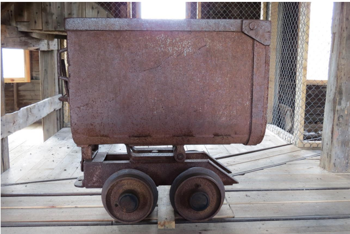
Right of Way mine – No 2 shaft – Side view of Wabi one-ton ore car. Dump door is on the right hand side; pivot point is just above and behind the right hand wheel. Sloping frame at right hand side prevents car body from over-tipping.
