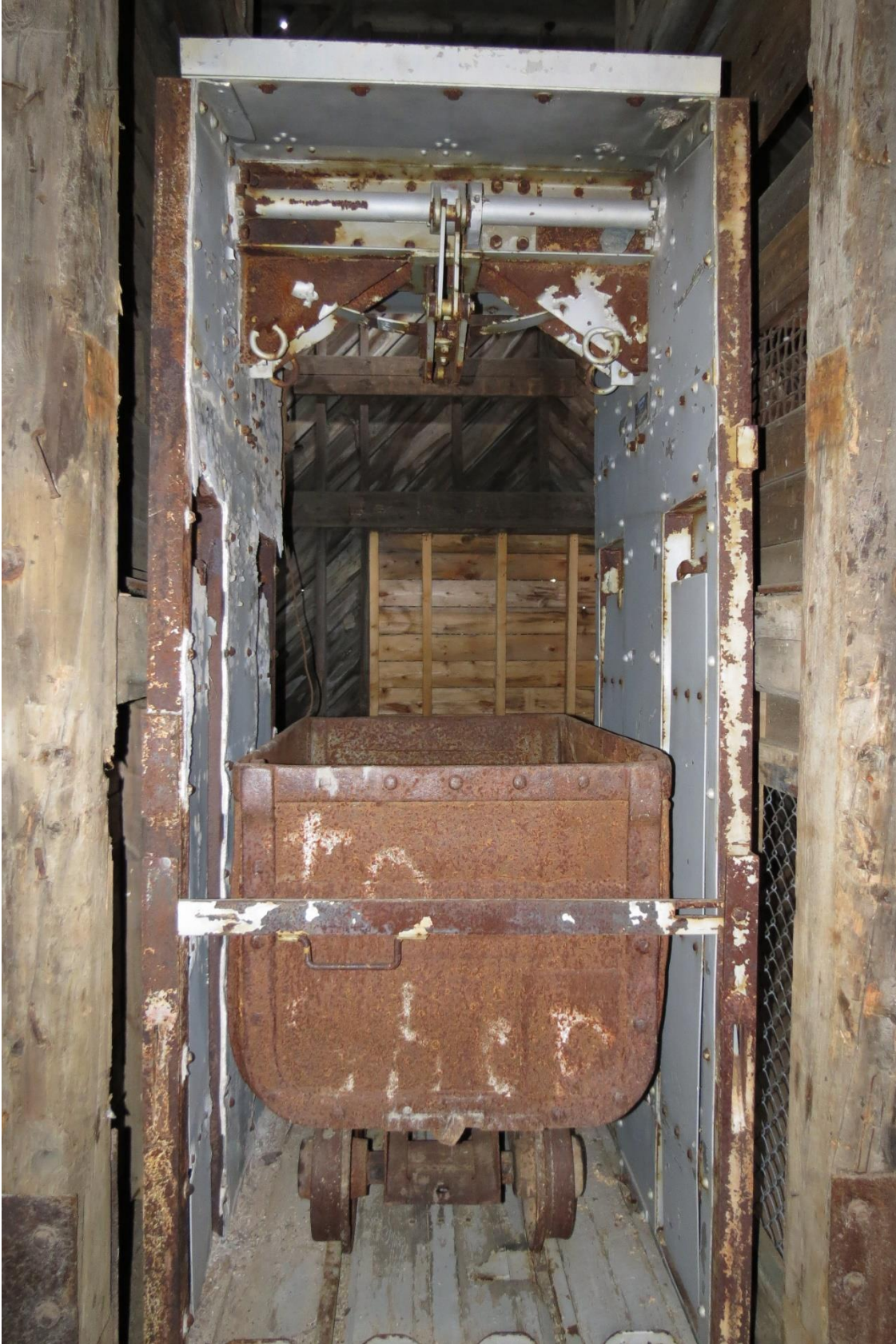
Right of Way mine – No. 2 shaft (cage and mine car)
