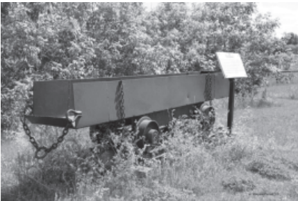
Drill steel car
